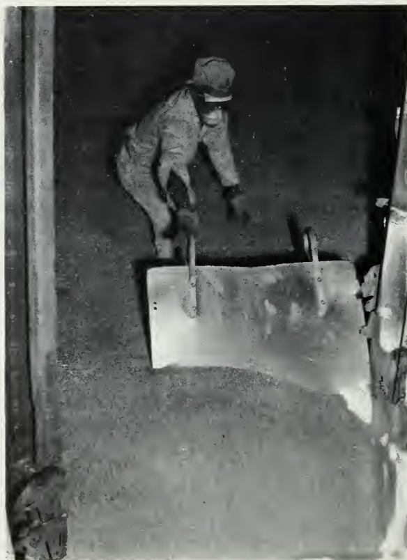
Figure 5.--Unloading a boxcar of grain by the power shovel method. The second worker and shovel are out of view.
