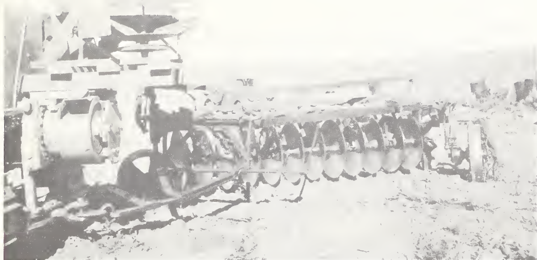
Figure D-11. --Gasoline-powered broadcaster mounted on a tractor to sow ahead of a wheatland-type plow.
