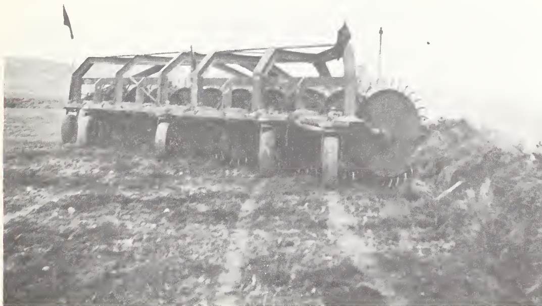
Figure A-19. --Rotary brush rake at work. (Photo by Bureau of Land Management.)
