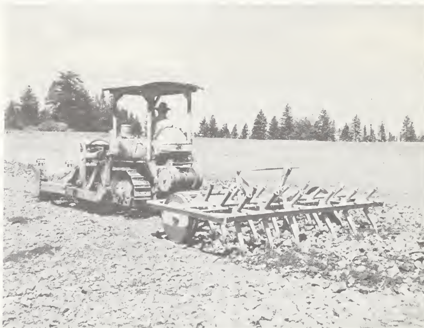
Figure A-15. --Rockland tiller in operation during spring on site typical of that for which it was designed.
