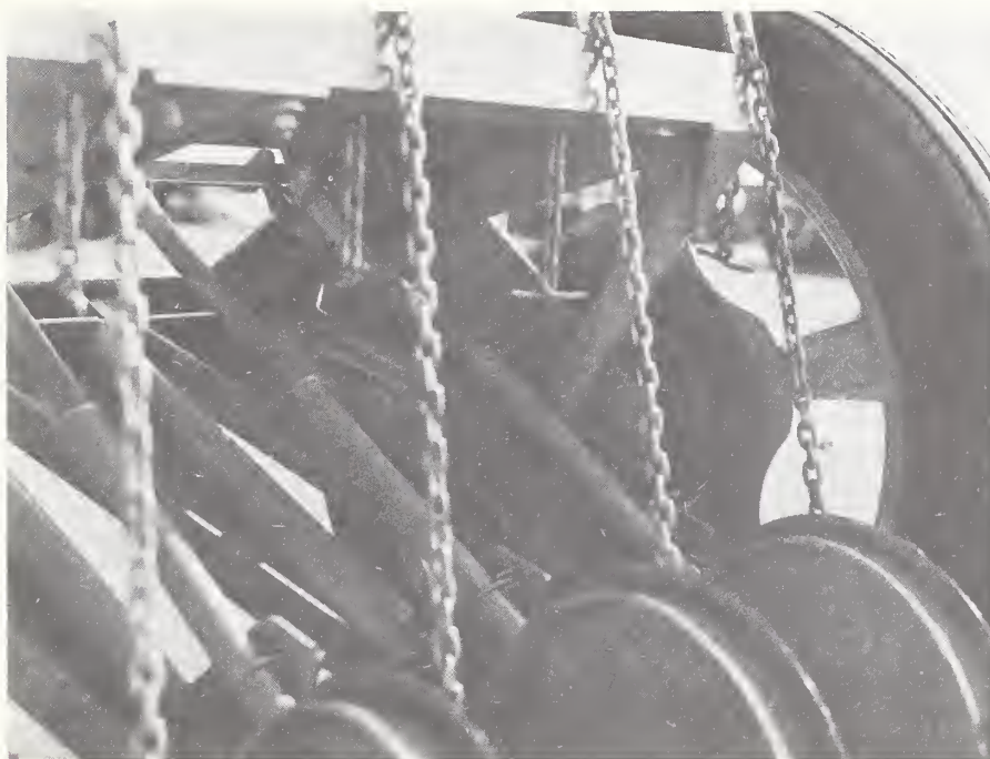
Figure D-6. --Close-up of rangeland drill mechanism showing disks, depth regulators, and seeding tubes. Each disk operates independently.
