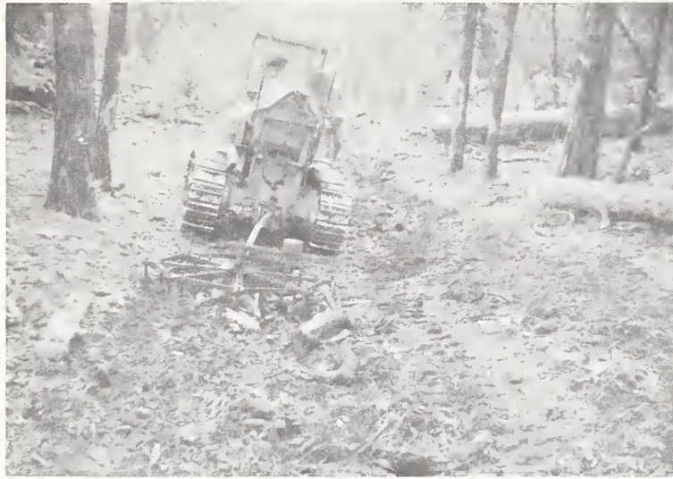
Figure F-1. --Rotary harrow in use on skidroad.
