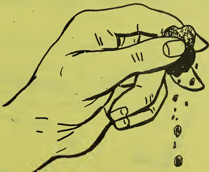
Method of crumbling soil between fingers
