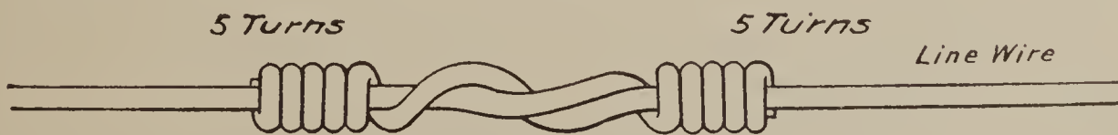
FIG. 5.—Method of joining wire.
