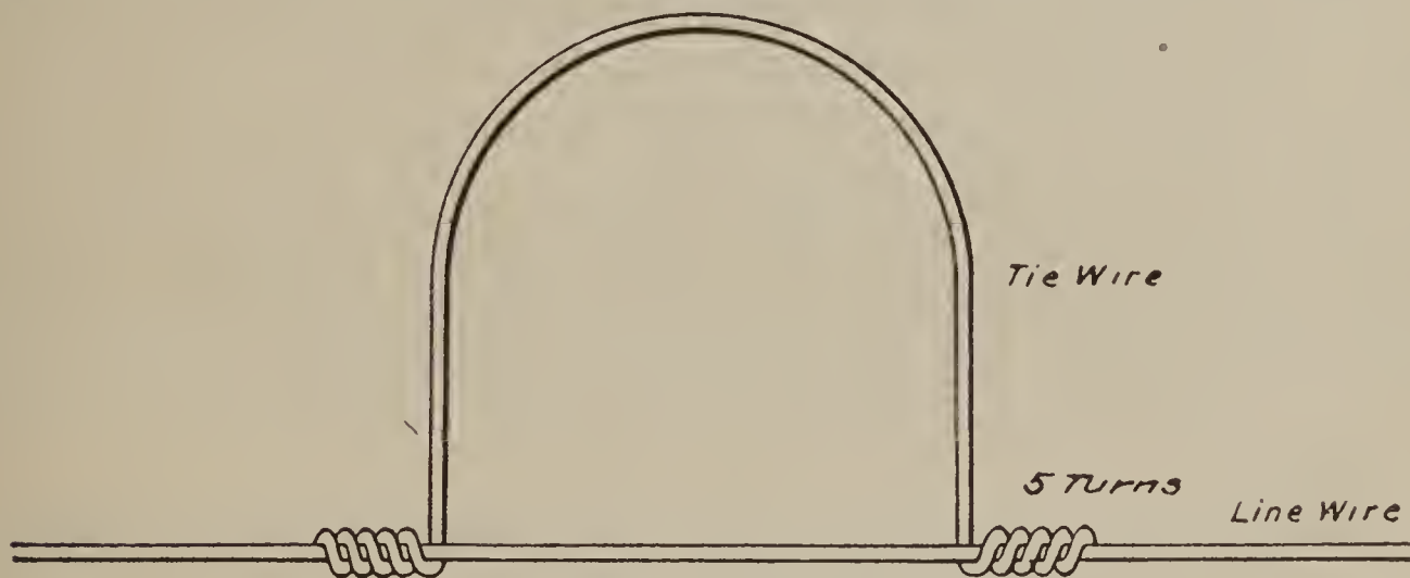
FIG. 4.—Method of tying wire to insulator.
