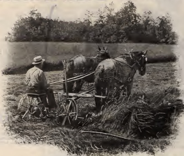
TWO HORSE FIVE-FOOT STANDARD WORCESTER MOWER. The photograph shows it, cutting double or back swath.
