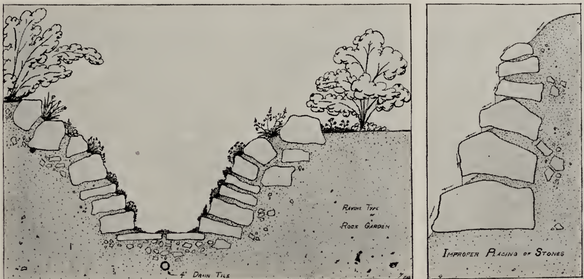
The right way to place stones in a rock garden (left), The wrong way is shown at the right.
