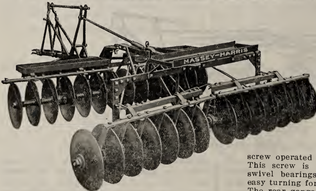
Sizes 6 feet, 7 feet and 8 feet, with either 16-inch or 18-inch discs.
