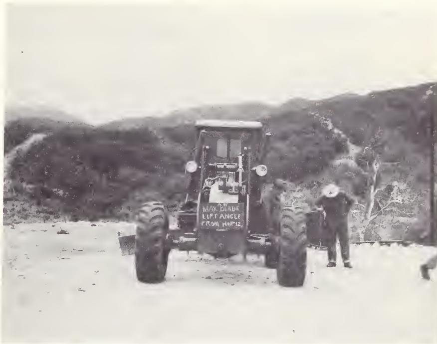
Fig. 10. Blade lift angle from centered position.
