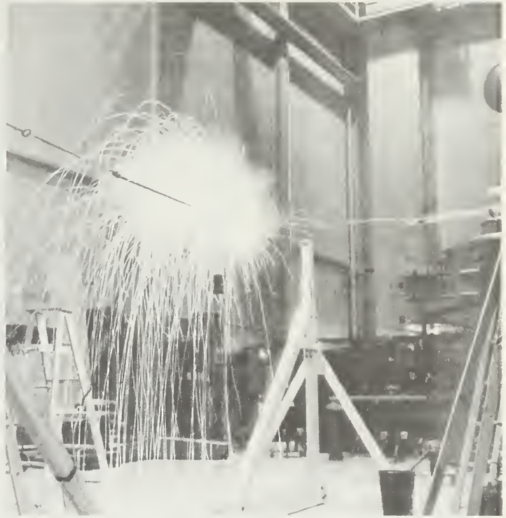
The effect of a high voltage power line falling on telephone cable is simulated in the laboratory to test the effectiveness of borrowers' station protector equipment.
