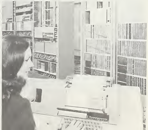
Changes in subscribers' service requirements can be made electronically, thus eliminating tedious hand labor. The entire program is stored electronically, ready to be altered instantly whenever changes are required.
