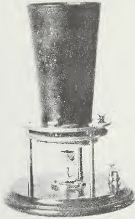
Bell's first telephone used sulphuric acid as part of its transmission apparatus. Its receiver was a tuned reed.
