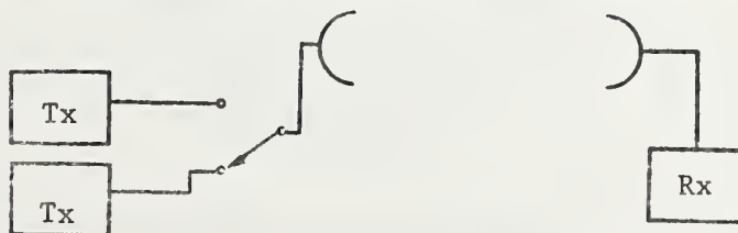
Figure II-18 Hot Standby Transmitter Configuration
