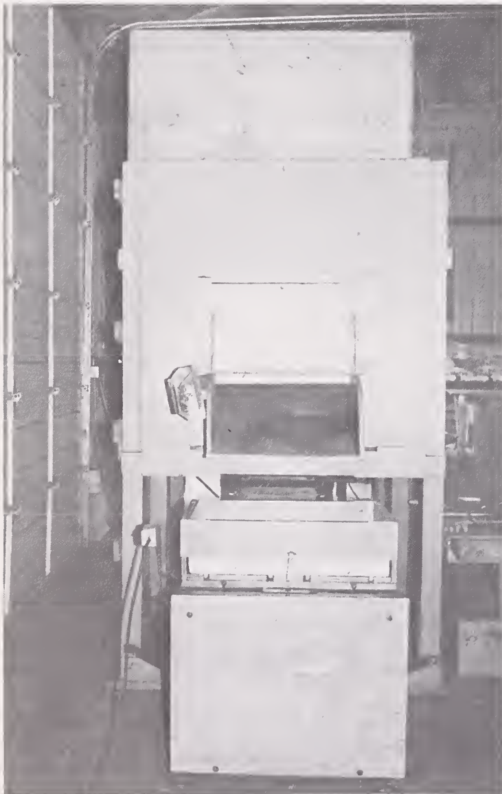
Figure 7-2.—Hopper used to dispense pot mix into containers.
