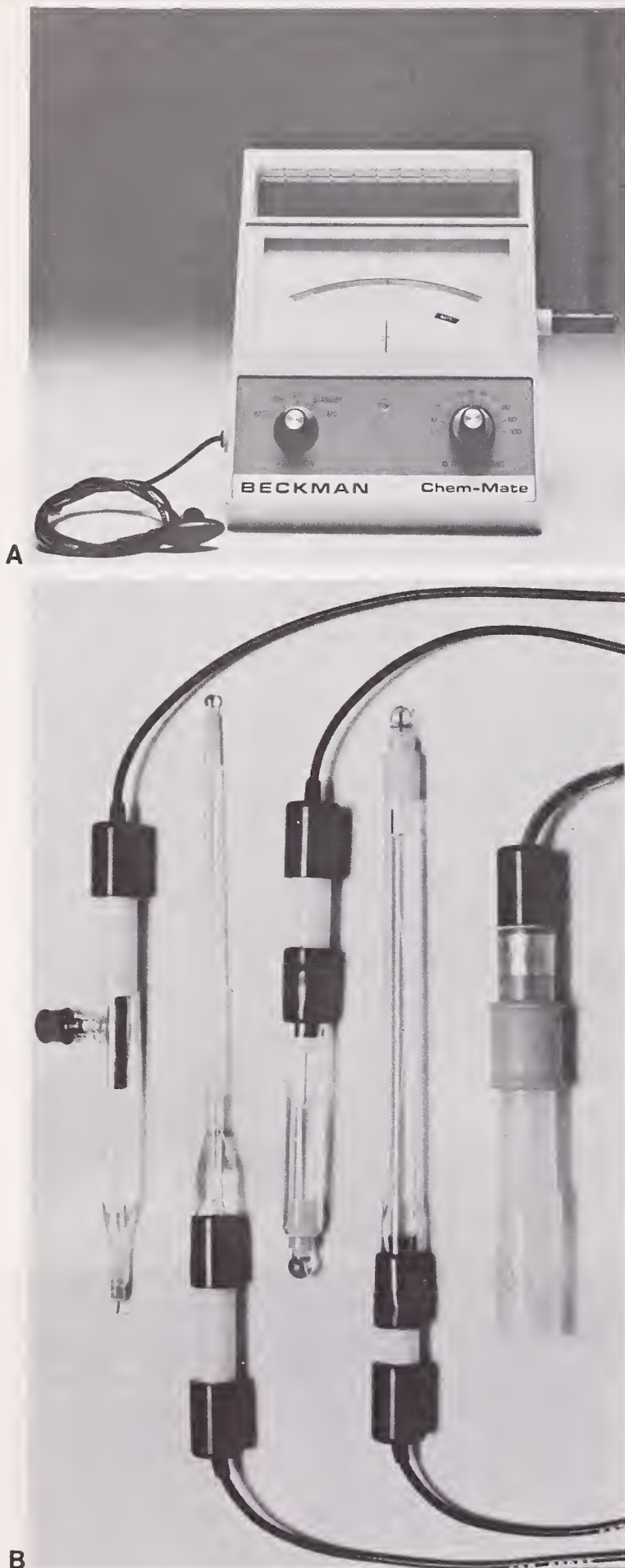
Figure 6-37.—Portable pH meter suitable for greenhouse use (A), and commonly used electrodes (B). (Photos courtesy of Beckman Instruments Co.)
