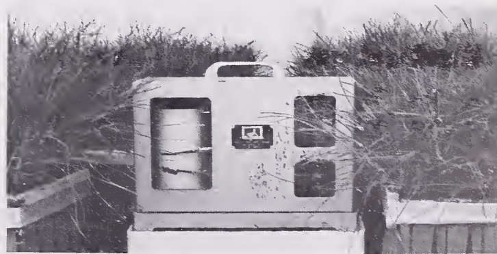
Figure 6-36.—A hygrothermograph is an essential greenhouse instrument which should be set at plant level, but may or may not be in a shelter.
