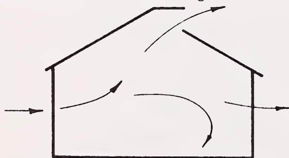
Figure 6-2.—Natural ventilation (Ekblad 1973).
