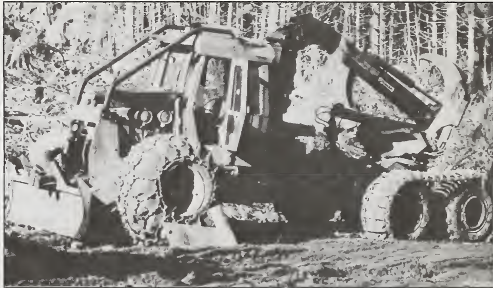
Figure 4—Forwarders that move large loads of small stems enhance the efficiency of harvesting dense stands.
