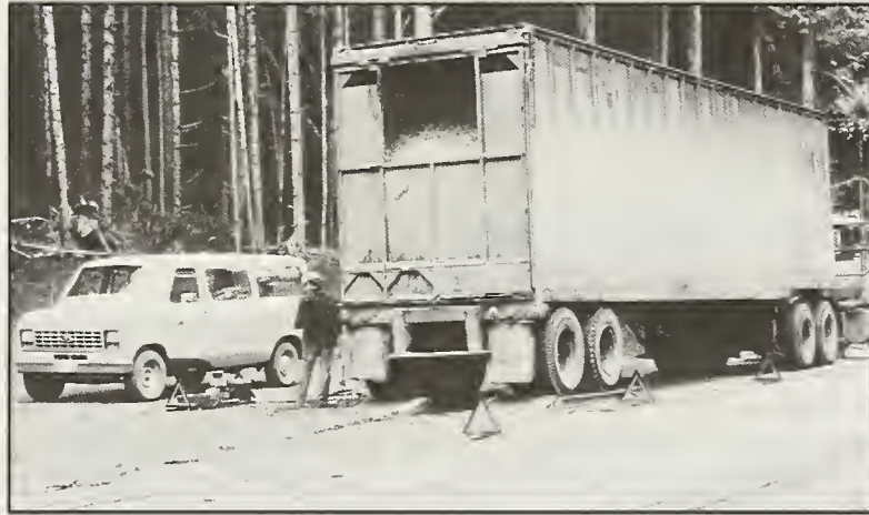
Figure 12—Total green weight of all products was found by weighing all trucks on portable scales.
