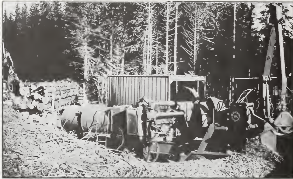
Figure 8—The chipper produced clean chips from stems that had been debarked and delimbed.
