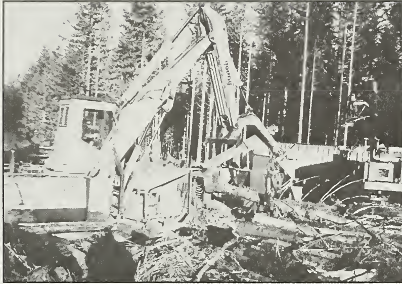
Figure 6—The mobile loader, which handles all materials arriving at the landing.
