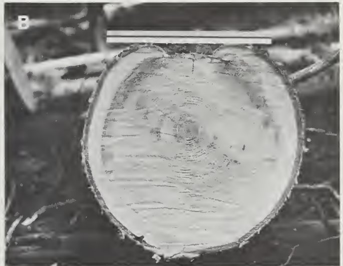
Figure 2.—A. Decay behind 14-year-old basal wound (left section) and 3 feet above wound (right section). B. Decay behind 14-year-old upper-bole wound. Scale is 12 inches.
