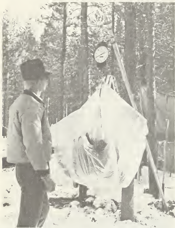
Figure 3.—Method of obtaining green weight of all branches in a crown section.
