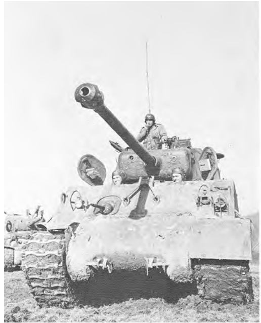
M4A3 SHERMAN TANK WITH 76-MM. GUN
