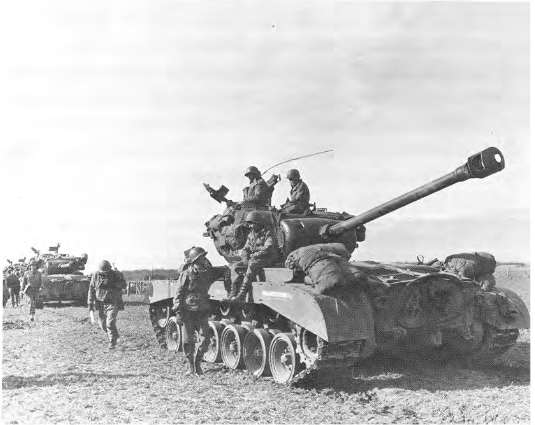
PERSHING TANK T26 WITH 90-MM. GUN
