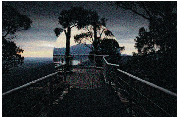
A simulation of an EVF view in low light (central portion magnified to aid manual focusing)
