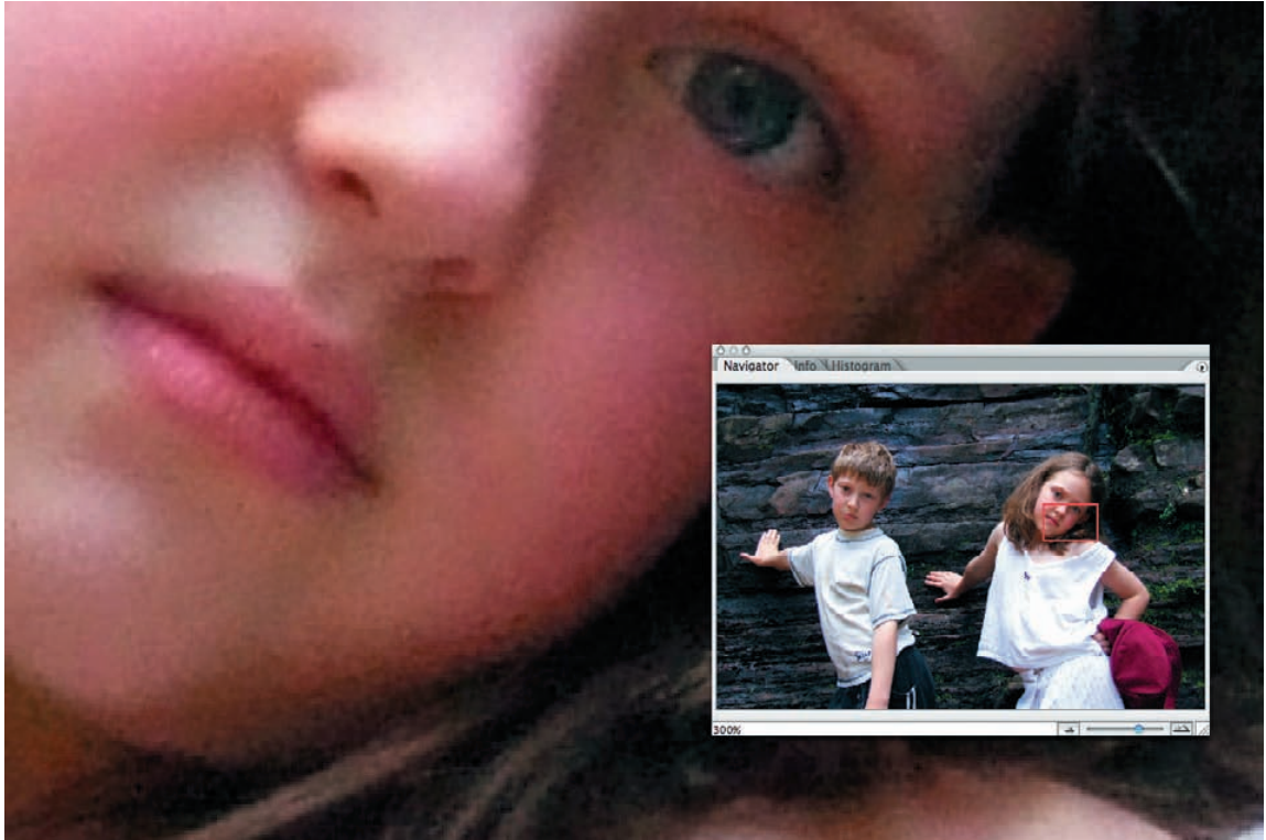
The small sensor of the s9500 pushes its luck at 400 ISO - image magnified to 300% (see inset)
