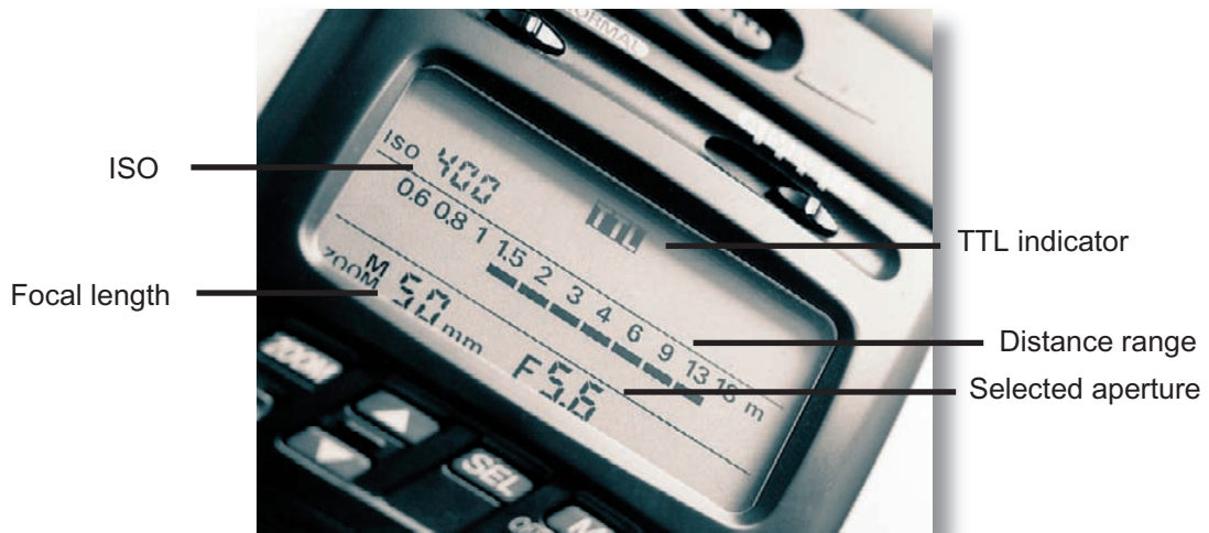
Control panel of a modern dedicated flash unit
