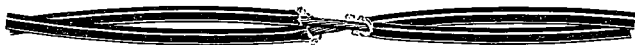
A SHORT CIRCUIT-TWO WIRES OF A PAIR IN CONTACT WITH EACH OTHER.
