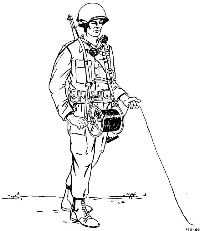
Figure 47. Recovering wire with Reel Equipment CE-11.
