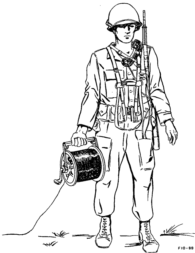
Figure 46. Laying wire with Reel Equipment CE-11
