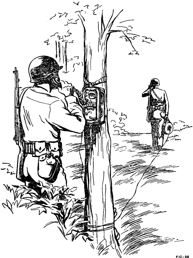
Figure 39. Paying-out field wire, using Wire Dispenser MX-306A/G.
