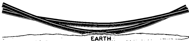
C GROUNDED CIRCUIT - ONE OR BOTH WIRES OF A PAIR IN CONTACT WITH A GROUNDED OBJECT.
