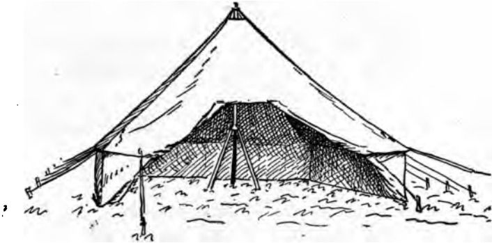
Fig. 29.—Pyramidal tent, with tripod support (United States Army standard model for fixed camps).
