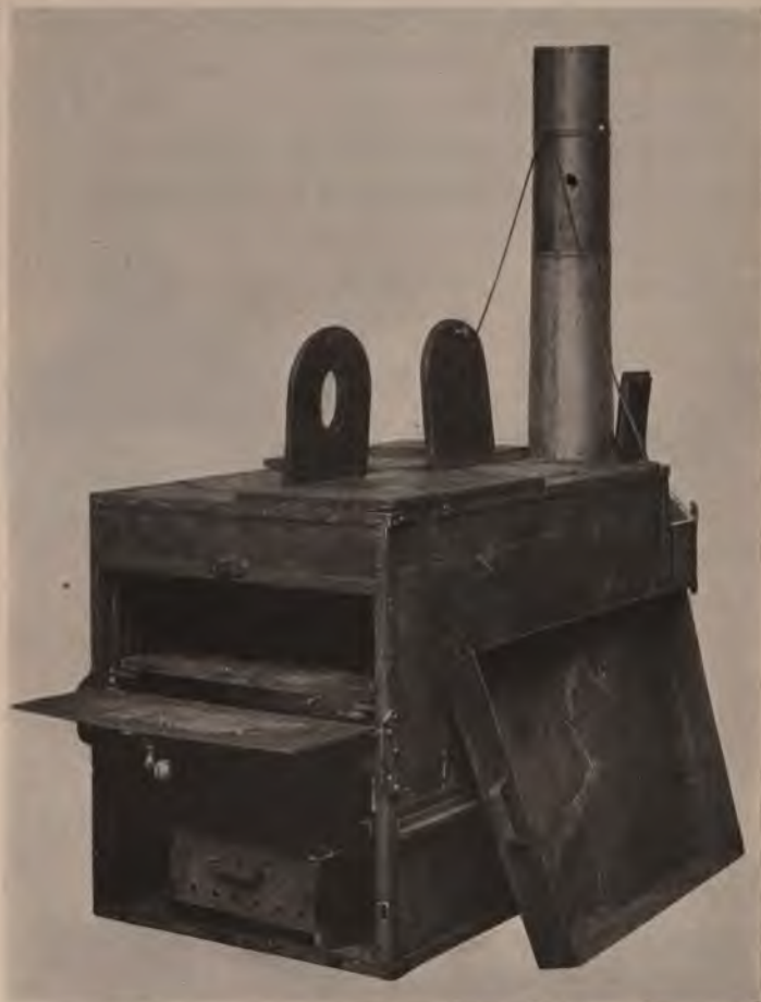
Fig. 40.—Incinerator for excreta, Quartermaster Corps type.
