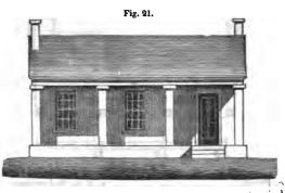
Figures 21 and 22, show the elevation and groundplan of a cottage, in which the rooms are rather more agreeably arranged, than in the former plan. The elevation, (Fig. 21,) has a piazza, running across the whole front. This would cost nearly two hundred dollars; and, for this sum, another story might be added. An architect told the writer, that he could build
