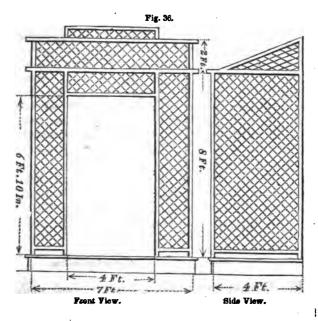
Fig. 36, is a latticed portico, which is cheap, and answers all the purposes of a more expensive one. It should be solid, overhead, to turn off the rain, and creepers should be trained over it. A simple latticed 24 p. E.
