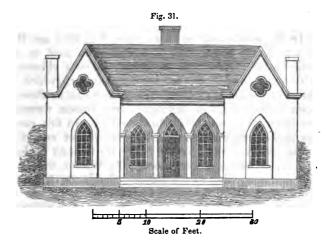
The elevation, (Fig. 31,) exhibits the front view. It has a recess in the central part, under which, is the door, with a window on each side of it. This forms a piazza; and into this, and a similar one at the back of the house, the two centre parlors open.
