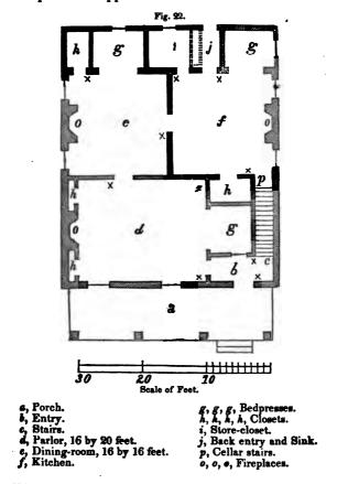
The parlor, d, is designed to have the doors (shown in Fig. 19) placed at the end, where is the bedpress, g. This will make it a handsome parlor, by day, and yet
