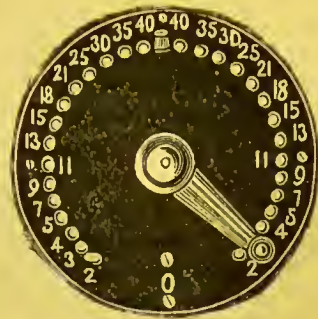
Dial collector arranged for starting from either end of the battery.
