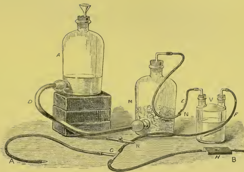
FIG. 5.—Carbonic acid apparatus. A. Bottle containing hydrochloric acid. M. Bottle containing fragments of marble on a stratum of broken glass. V. Wash-bottle. H. Object support, fig. 16. G. T-tube which communicates with the gas apparatus by the tube F, which is guarded by a clip, and in the opposite direction with H. By its stem it is in direct communication with the mouth of the operator by a tube on which there is also a clip. When the first clip is closed, carbonic acid collects in M and drives back the hydrochloric acid into A; a current of air can then be drawn through G and H. If the clip on the mouth-tube is closed and that on F opened, carbonic acid passes through H. p. 16.
