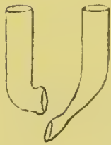
FIG. 218.—Cannulae for aorta and vena cava of frog. The right-hand figure represents the arterial cannula. They are of size suitable for large specimens of R. esculenta (§ 46).
