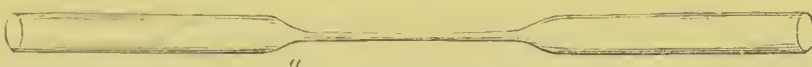
FIG. 327.—A tube drawn out in order to seal it. The operation is completed by directing the point of a blowpipe flame on the point a , and drawing the two ends of the tube rapidly apart.
