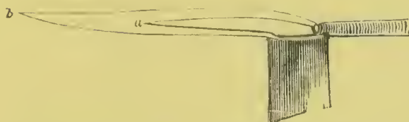
FIG. 325.—Blowpipe flame. a , reducing, b , oxidizing part of the flame.
