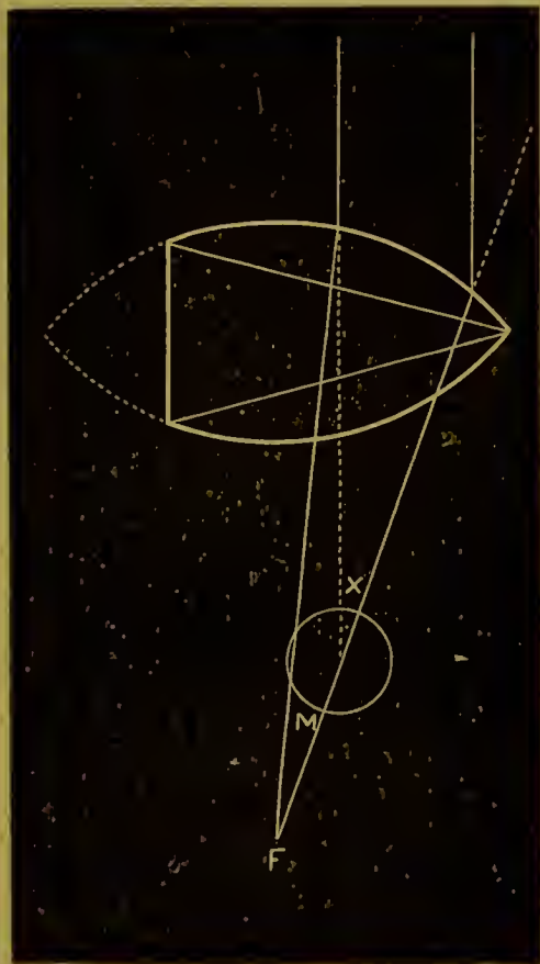
FIG. 3.—The position of the prism does not affect the result, even if it is put inside the lens, as in a prismosphere the deviating effect is the same. The angle X has the same magnitude as in Fig. 2.
