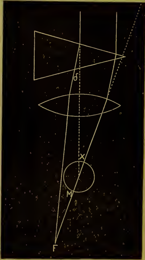
FIG. 2.—Parallel rays of light on traversing the prism as before undergo a deviation \delta . On reacting the lens, since the pencil of rays is oblique, they will converge to the (secondary) focus F , which is not on the principal axis. The visual line must consequently undergo a deviation X . The ray of light which it receives on its macula passes through an eccentric portion of the lens, which therefore acts as an additional prism. Accordingly in this case X is greater than \delta .
