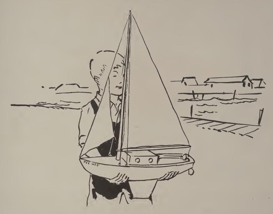
When Mate had time to fit out his ship model, he set up his round mast with wires to keep it up. He made a sail from an old handkerchief. He used string instead of rope. He used little screw eyes in place of pulleys and fittings.
