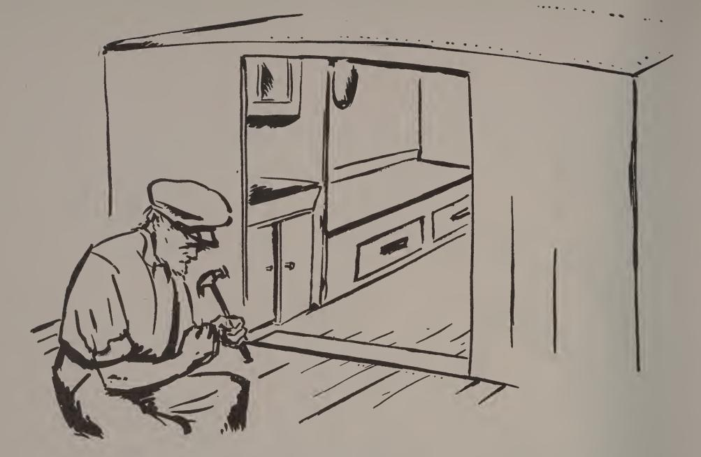
While the men sanded the outside of the hull, Captain began work on the inside. He laid the floor in the cabin and in the cockpit aft of the cabin. The cockpit is the inside of the hull not covered by a roof or deck. He built bunks in which to sleep, and a little galley, or kitchen. He built a toilet, and lockers in which to put clothes and food.
