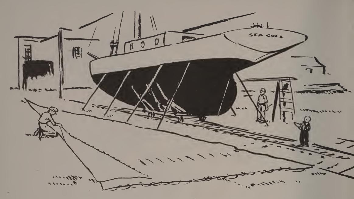
The large sail was called the MAINSAIL, and the small one the JIB. The mast was fitted with a long pole called a BOOM to hold the bottom of the sail in position. The mast was held straight by wires. The sails were spread out near the boat and fitted with ropes and mast rings. The large lead keel was now bolted to the bottom of the boat.
