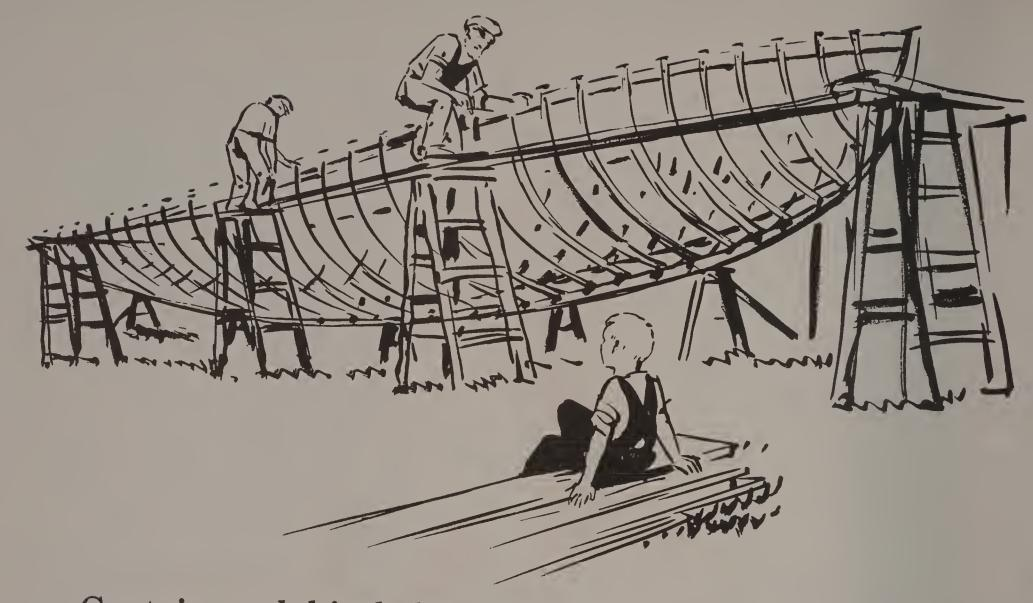
Captain and his helpers bent a heavy piece of wood along the ends of the ribs. This is called the SHEER. Each rib was fastened to the sheer. Captain bolted several long boards to the inside of the ribs. He also bolted a heavy beam on top of the keel. It held the ribs secure and strengthened the boat. Then they began to plank the boat. Each plank must be shaped to fit exactly.
