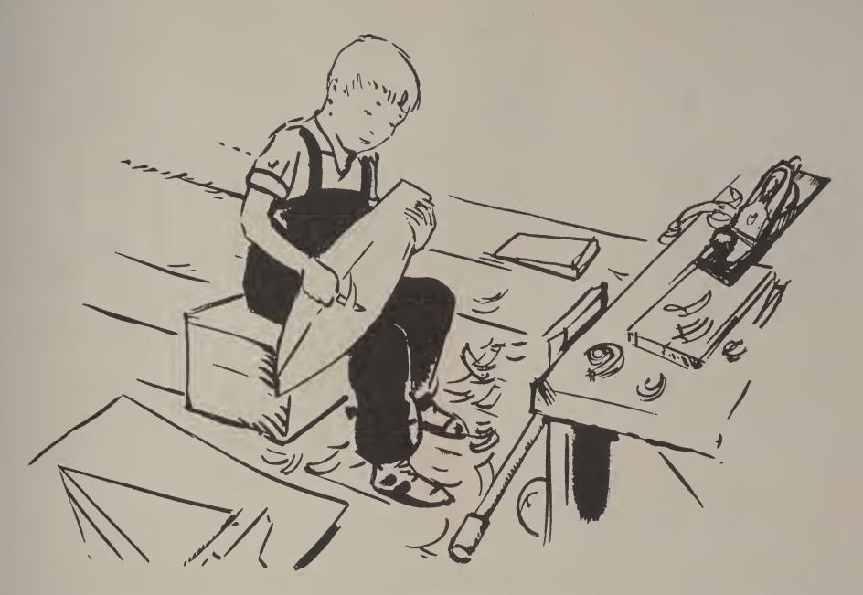
The part of the boat that floats in the water is called the HULL. Mate used his plane to shape the hull of his boat. He also used his jackknife. He knew the boat must balance in the water. He was careful to plane both sides of the hull the same.
