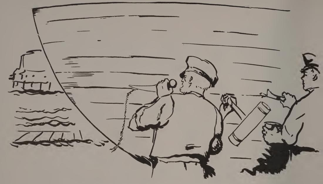
Next time Mate came to the shipyard there was a ringing sound like many hammers striking a bell. Mate found Captain and his helpers caulking the boat. A long thread of candlewicking was pressed into each seam. Then this was driven in with a caulking iron and mallet until the seam was almost filled. Over this, white lead was spread until the seam was full.
