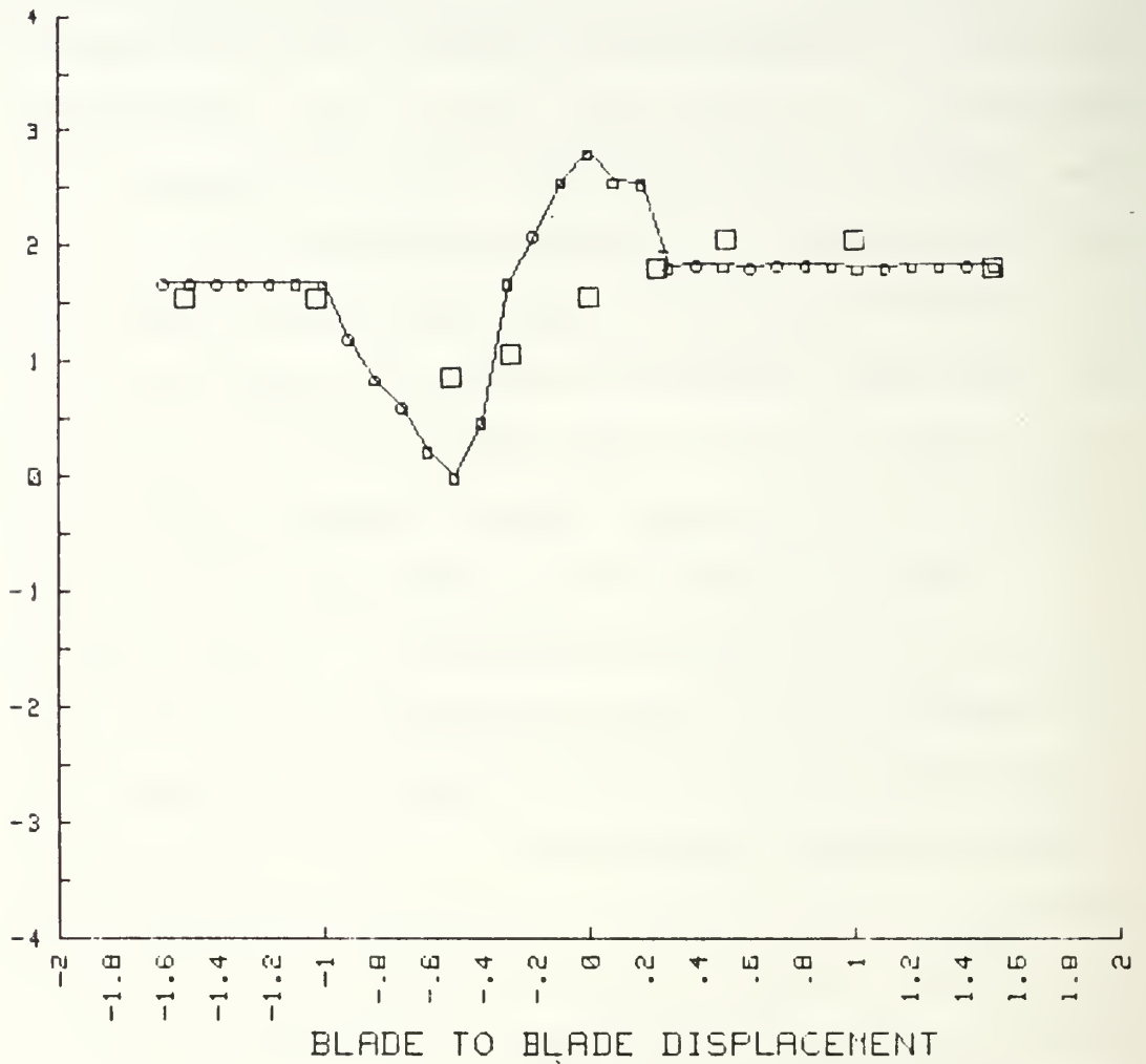
Figure 13. Outlet Air Angle Vs Blade to Blade Displacement at Station 2-6 for \beta_1=40.3^\circ . (US Corp. 5 hole cylindrical probe and yaw probe.)
