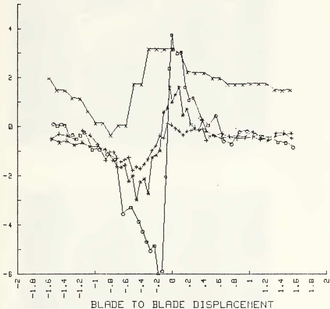
Figure A32. Comparative Plots of Beta2 Vs Blade to Blade Displacement. (Angle measurements corrected to average yaw probe reading at station 2-6 on pressure side of blade.)
