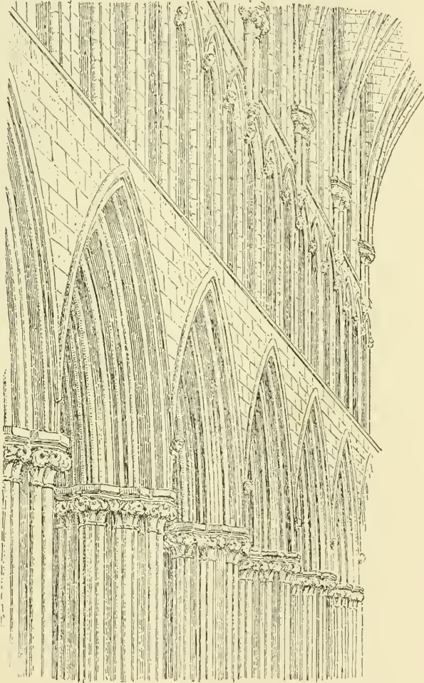
FIG. 120.—System of Nave of Wells.
