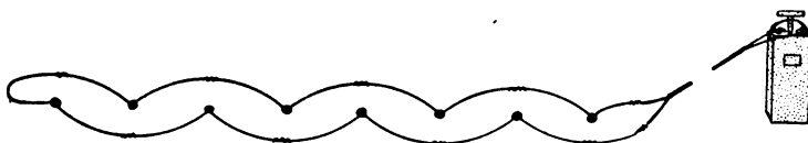
ANOTHER METHOD OF CONNECTING DUPLEX LEADING WIRE
