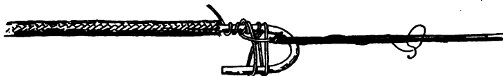
AN EXCELLENT METHOD OF CONNECTING AN ELECTRIC BLASTING CAP WIRE TO A LEADING WIRE
