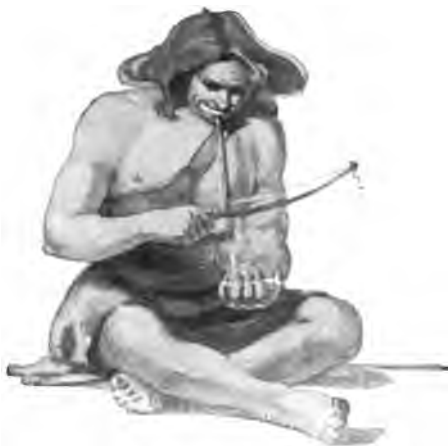
A drill for boring holes can be made into a fire drill
