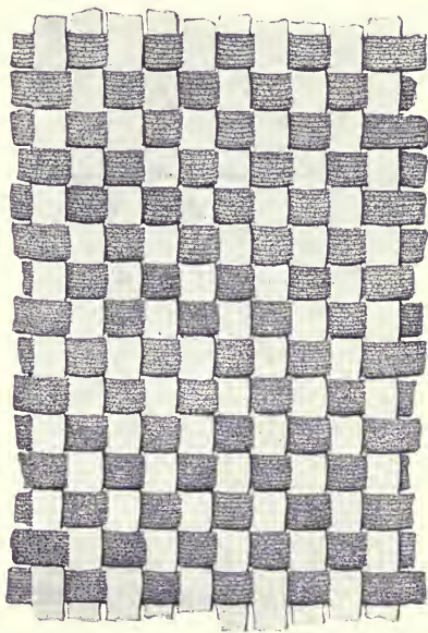
"At first they wove each woof strand under and over each strand of the warp"
