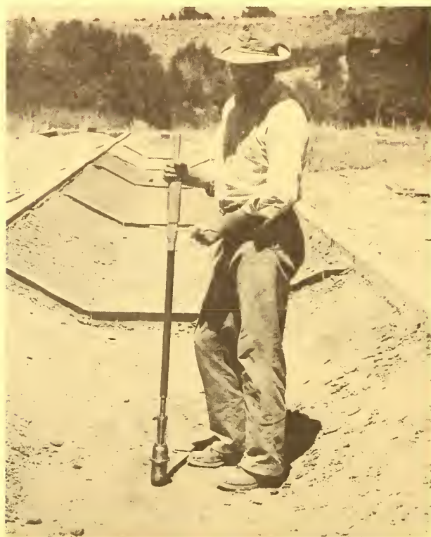
FIGURE 5. — Coring device used to obtain samples for apparent specific weight determinations.
