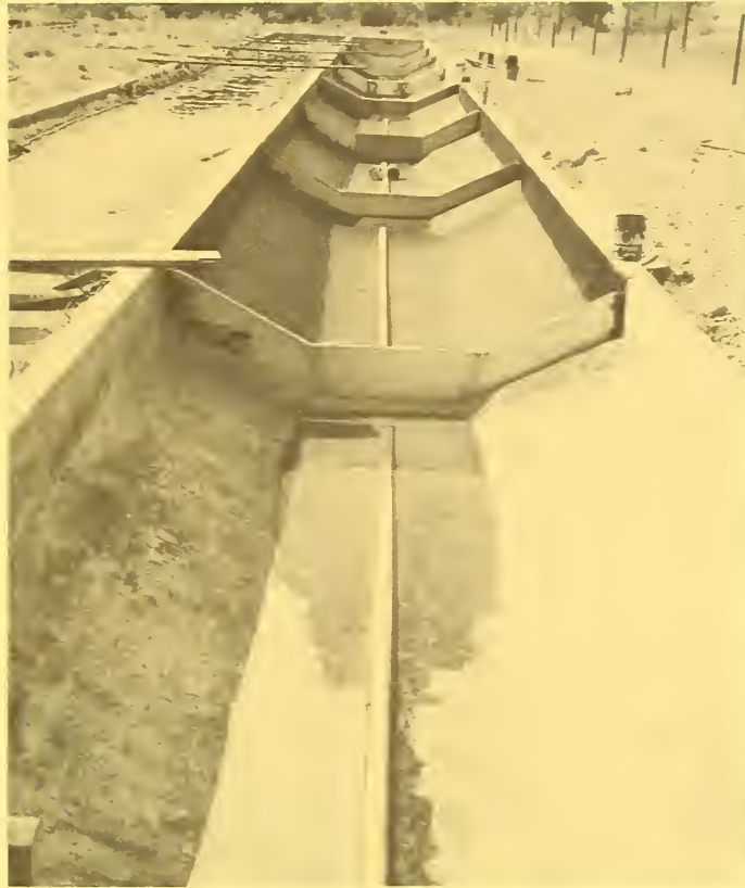
FIGURE 3. — Experimental seepage-control channel before addition of subgrade material. Metal dividers are already sealed in place in the concrete basin.
