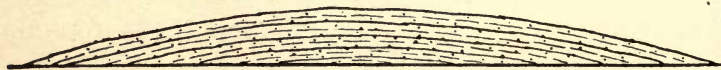
FIG. 13. SECTION THROUGH THE ISLAND SHOWN IN FIG. 12. Slopes of surface coincide with arrangement of strata.
