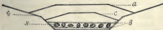
69. Simple form of germinator. G, soup-plate; B, cloth or blotting-paper; H, seeds; C, saucer inverted; A, small dinner plate inverted. Note.—The cloth (B) must not project outside of C, because of the drying effect of the air and the capillary attraction of the cloth.
