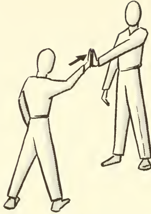
FIG. 30. An experiment to show that with a given energy you can either slowly exert a large force through a small distance or rapidly exert a small force through a large distance. This is demonstrated by having your partner offer either a large or small resistance to your push.
