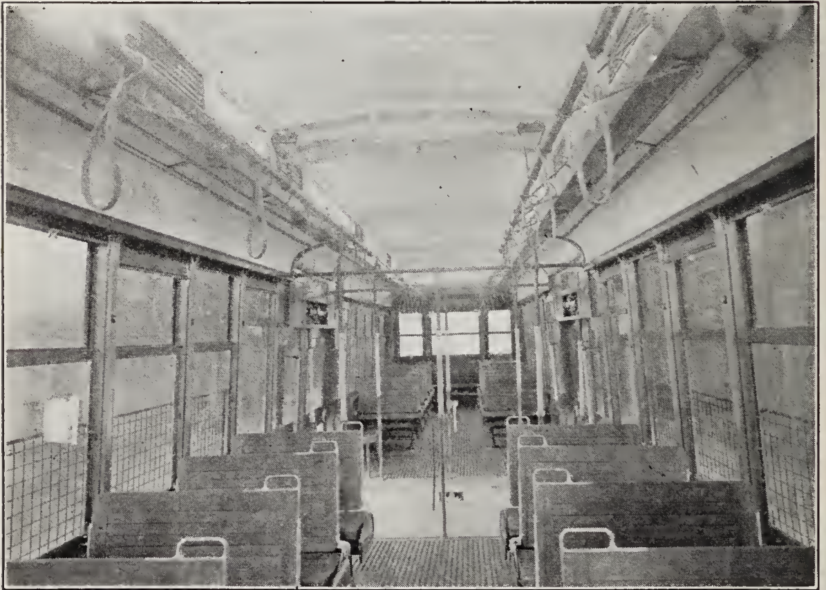
FIG. 358. — Large semi-convertible prepayment car with powerful motors. The center entrance makes this car also convenient to use as a trailer.
