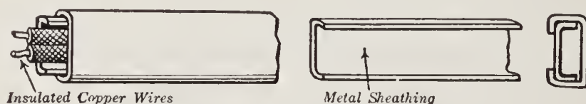
FIG. 310. — National metal molding.
