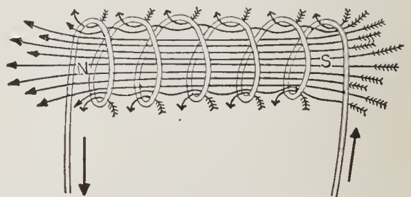
FIG. 49. — Loose solenoid with its lines of force.
