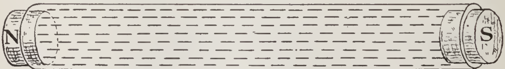
FIG. 75. — Glass tube of steel filings after magnetization.
