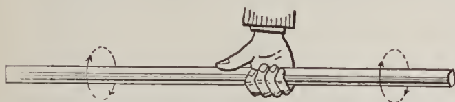
FIG. 47. — Thumb rule for magnetic field around a wire.
