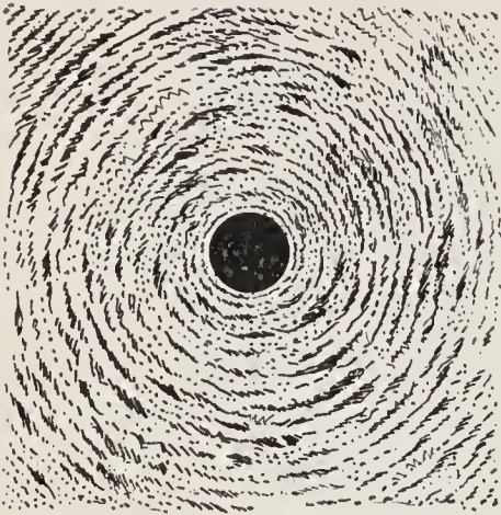
FIG. 44. — Iron filings showing the distribution of magnetism around a wire carrying an electric current. The black dot represents a cross section of the wire.
