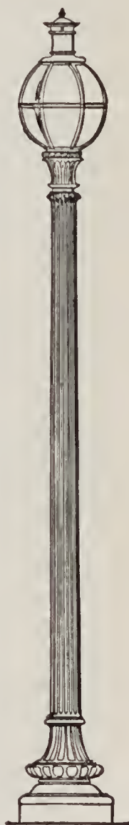
FIG. 335.—Ornamental type of diffusing globe and pole used in Washington, D. C.
