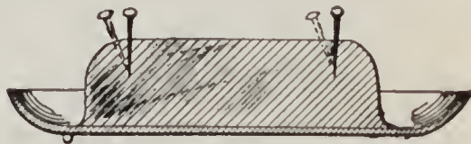
FIG. 391. — Jelly analogue of electromagnetic induction.
