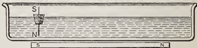
FIG. 41. — Experiment to illustrate the movement of a free magnet pole when near a bar magnet.
