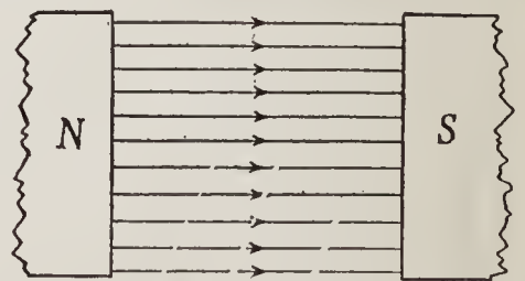
FIG. 163. — Uniform magnetic field.
