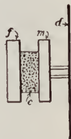
FIG. 374. — Principle of carbon transmitter.
