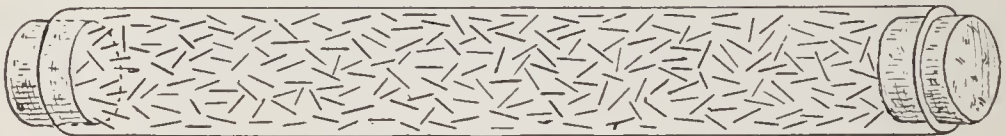
FIG. 74. — Glass tube of steel filings before magnetization.
