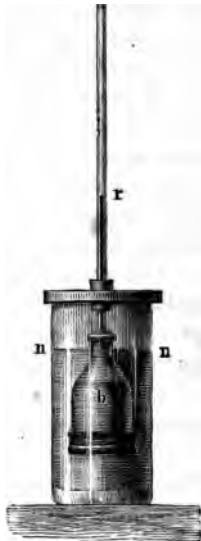
FIG. 61.—Apparatus for measuring osmose: b , a vessel filled with cupric sulphate closed below by a permeable membrane, and placed in a vessel of water. As the water passes through the bladder to mingle with the cupric sulphate, the level of the fluid will rise in the tube r in connection with the vessel b , but will fall at n , in the outer vessel.
