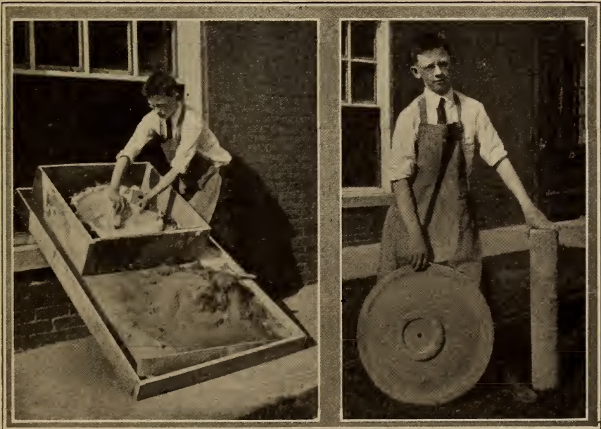
Illus. 22. Using the Sweep on a Plaster of Paris Form Preparatory to Casting the Top of a Bird Bath. Illus. 23. Completed Top of Bird Bath and the Shaft.
