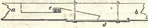
Fig. 89—Represents a scarf joint arranged to resist a cross strain and one of extension. The bottom of the joint is secured by an iron plate confined by bolts. The folding wedge key inserted at c serves to bring all the surfaces of the joints to their bearings.
