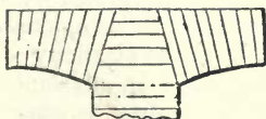
Fig. 47—Represents a mode of arranging the voussoirs and horizontal courses in flat segment arches.
