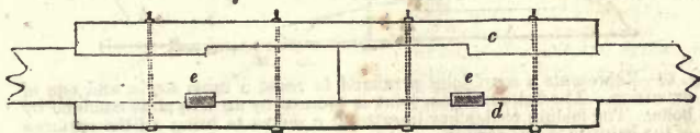
Fig. 86—Represents a fished joint in which the side pieces c and d are either let into the beams or secured by keys e , e .
