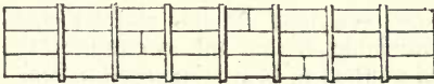
Fig. 57—Represents a solid built beam of three courses, the pieces of each course breaking joints and confined by iron hoops.
