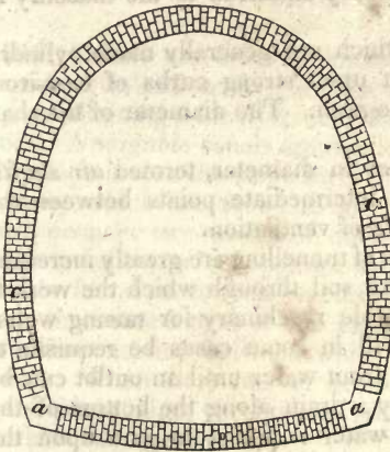
Fig. 163—Represents the general form of the cross section c of a brick arch for tunnels.
