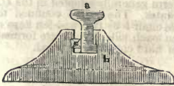
Fig. 157—Represents a cross section a , of the fish-bellied rail of the Liverpool and Manchester Railway, and the method in which it is secured to its chair. The rail is formed with a slight projection at bottom, which fits into a corresponding notch in the side of the chair b . An iron wedge c is inserted into a notch on the opposite side of the chair, and confines the rail in its place.
