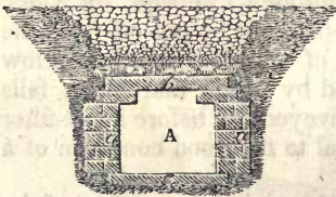
Fig. 155—Cross section of a covered drain.
