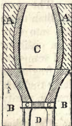
Fig. 1 represents a vertical section through the axis and centre lines of the entrances communicating with the interior of a kiln for burning lime with coal.
