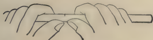
FIG. 3.— Breaking a piece of glass tubing. Make a scratch on one side of the tubing with a single stroke of the file. Place the thumbs on the other side of the tubing, directly opposite the file mark. Grasp the tubing with the thumbs and press backwards towards the thumbs.
