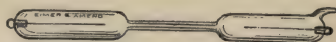
FIG. 35. — A form of tube in which gases are electrically heated to incandescence.
