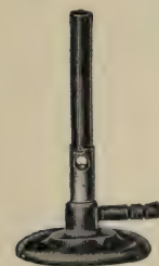
FIG. 1. — Bunsen burner . Ordinary form for use with coal gas.
