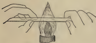
FIG. 4. — Drawing out glass tubing.
