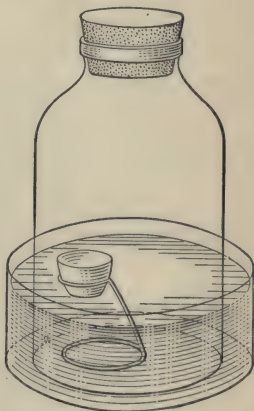
FIG. 24. — Apparatus for Experiment 27. Removing the oxygen from the air by burning phosphorus.
