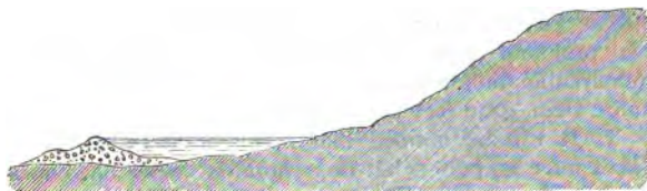
FIG. 54.—Section of a lake dammed up by a barrier of earth or gravel.
