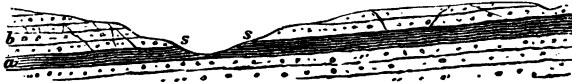
FIG. 43.—Section across a valley to show how the simplest kinds of springs arise.
