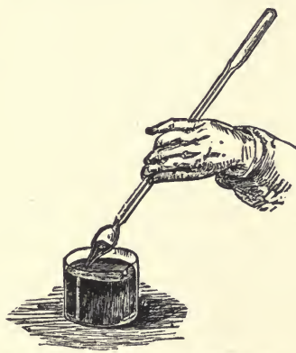
FIG. 5.—INTRODUCTION OF MERCURY.
