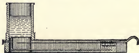
FIG. 30.—DINES'S HYGROMETER (SECTION).
