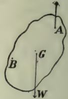
FIG. 17.—How to find the centre of gravity of a body of any form.
