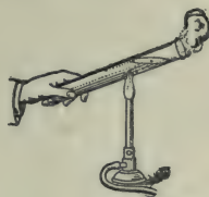
FIG. 163.—Water is a poor conductor of heat.
