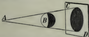
FIG. 182.—If the source be small the shadow will be sharp. A is the source, B the object, CD the shadow.
