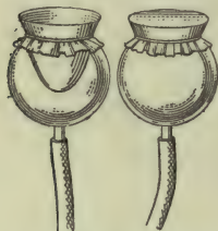
Fig. 72.—Rubber membrane forced inwards by pressure of the air.
