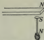
FIG. 225.—A nail if held near a magnet becomes itself a magnet by induction.
