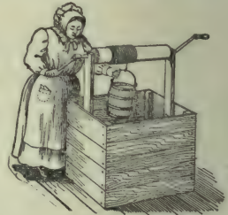
FIG. 49.—Windlass used in drawing water from a well.
