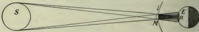
FIG. 184.—Showing how an eclipse of the sun is produced. A person at a cannot see the sun.
