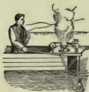
FIG 122a.—Apparatus for producing the sound, in Lake Geneva.
