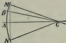
FIG. 193.—A section of a spherical mirror.
