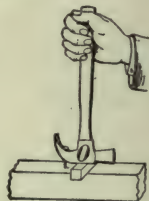
FIG. 31.—Claw-hammer, used as a lever of the first class.
