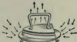
FIG. 170.—Convection currents in air about a heated flat-iron.
