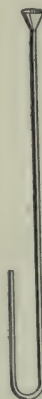
FIG. 82.—Air compressed within a closed tube by weight of mercury in the long branch.
