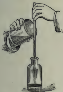
FIG. 115.—How to utilize surface tension in pouring a liquid.
