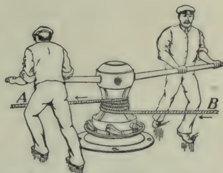
FIG. 50.—Raising the ship's anchor by a capstan.
