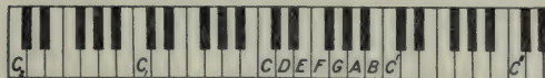
Fig. 125.—Central part of a piano key-board. The notes marked C_2 , C_1 , C , C' , C'' , go up by octaves.
