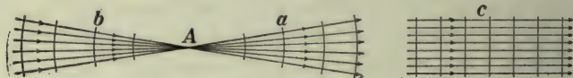
FIG. 180—A convergent pencil, b ; a divergent pencil, a ; a parallel beam, c .
