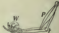
FIG. 38.—Human forearm, lever of the third class. One end of the biceps muscle is attached at the shoulder, the other is attached to the radial bone near the elbow, and exerts a force to raise the weight in the hand.
