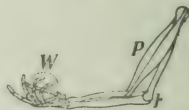
FIG. 38.—Human forearm, lever of the third class. One end of the biceps muscle is attached at the shoulder, the other is attached to the radial bone near the elbow, and exerts a force to raise the weight in the hand.
