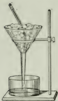
FIG. 147. — Determination of freezing point.
