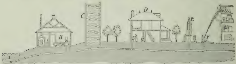
FIG. 62.—Water supply system. A , source of water supply; B , pumping station; C , stand-pipe; D , house supplied with water; E , fountain; F , hydrant for fire hose.
