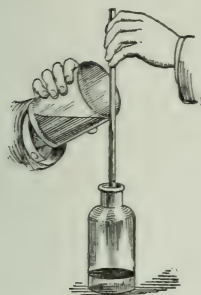
FIG. 115.—How to utilize surface tension in pouring a liquid.
