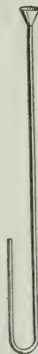
FIG. 82.—Air compressed within a closed tube by weight of mercury in the long branch.
