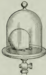
FIG. 83.—Expansion of air when pressure is removed.
