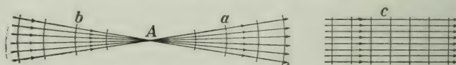
FIG. 180—A convergent pencil, b ; a divergent pencil, a ; a parallel beam, c .
