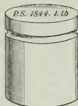
FIG. 4.—Imperial Standard Pound Avoirdupois. Made of platinum. Height 1.35 inches; diameter 1.15 inches. "P.S." stands for parliamentary standard .
