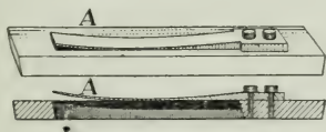
FIG. 133.—An organ reed. The tongue A moves in and out of the opening. This is called a free reed .
