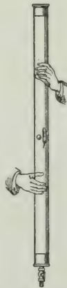
FIG. 10.—Tube to show that a coin and a feather fall in a vacuum with the same acceleration.
