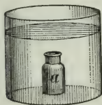
FIG. 105.—Copper sulphate solution in a bottle, placed in a vessel of water. In time the blue solution spreads all through the water.
