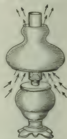
Fig. 177. — Air currents produced by placing a jacket around a heated body.
