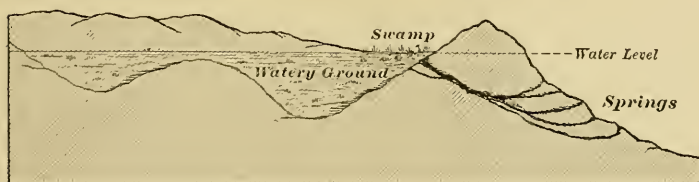
DIAGRAM SHOWING THE FLOW OF PERCOLATING WATERS
