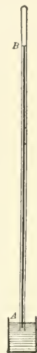
Fig. 221. — Diagram to illustrate the principle of the barometer. The pressure of the air at A maintains the mercury at B in the tube when there is no air in the tube above B .
