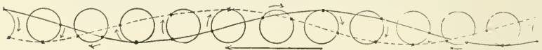
Fig. 154.—Diagram to illustrate the movement of water in waves. The small circles represent the movement of water particles.
