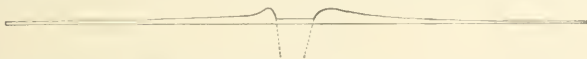
Fig. 88.—Levees of the Mississippi in cross-section, four miles north of Donaldsonville, La. Vertical scale \times 50 . The horizontal line represents sea-level. The bottom of the channel is far below sea-level at this point.
