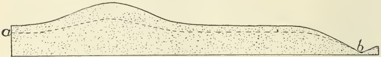
Fig. 21.— Diagram illustrating the position of the ground-water surface (the dotted line) in a region of uneven topography.
