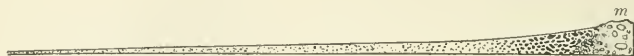
Fig. 133.— Diagram to illustrate the profile of a valley train, and its relations to the terminal moraine ( m ) in which it heads.
