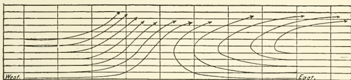
Fig. 242.—Diagram illustrating the general position of air currents in a cyclone of intermediate latitudes, and the fact that the upper air moves mostly toward the east, in the direction of the prevailing winds. (U. S. Weather Bureau.)
