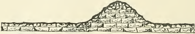
Fig. 121.— Diagram representing a hill unworn by ice, and the irregular contact of soil and rock.
