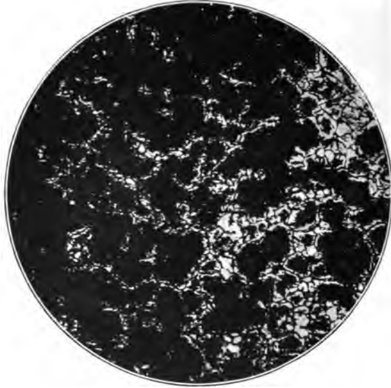
FIG. 63.—1·2 per cent. Carbon Steel (quenched from 700° C.). × 150.
