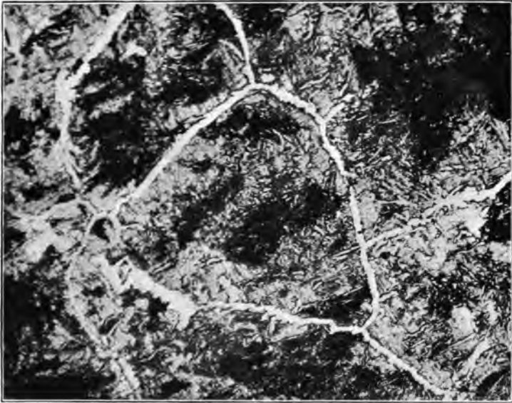
FIG. 28.—Converted Bar. Supersaturated steel. \times 58 .
