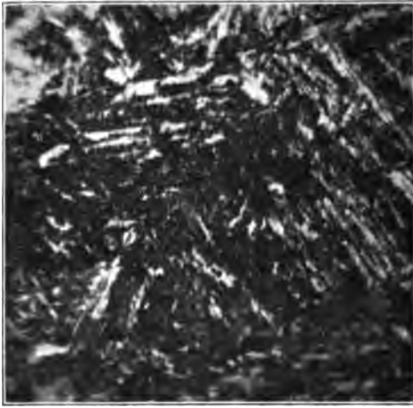
FIG. 61.—1·2 per cent. Carbon Steel (quenched from 800° C.). × 1000.
