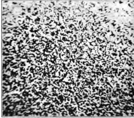
FIG. 44.—0.36 per cent. Carbon Steel (forged). × 58.
