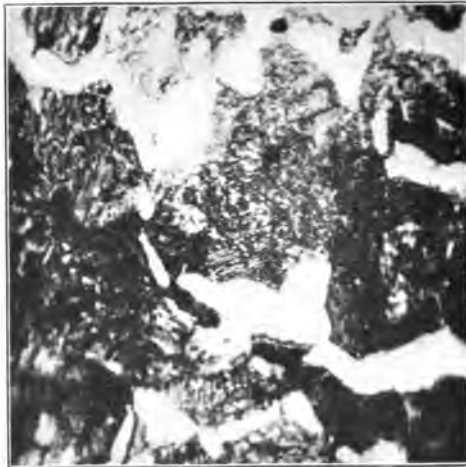
FIG. 64.—1·2 per cent. Carbon Steel (quenched from 600° C.). × 1000. [To face p. 243.]
