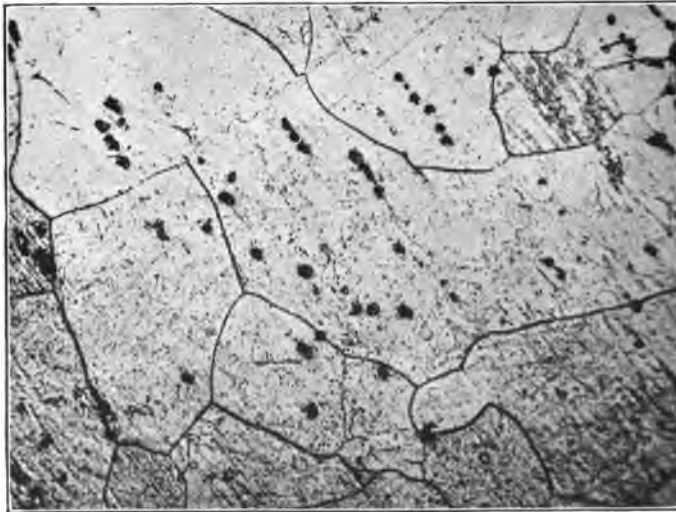
FIG. 45.—Ferrite (slowly cooled from 1000° C.). × 150. [To face p. 234.]
