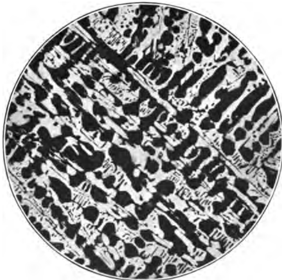
FIG. 29.—White Cast Iron. 3.4 per cent. carbon. \times 150 . [To face p. 166.]
