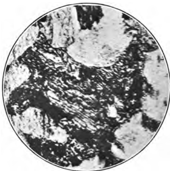
FIG. 60. Annealed Razor. \times 1000 .
