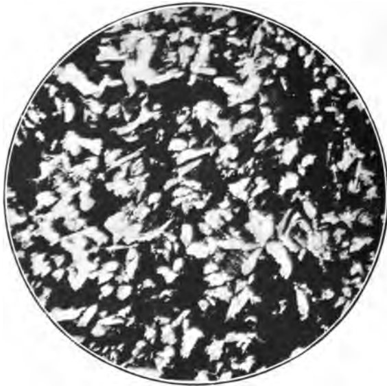
FIG. 42.—0.36 per cent. Carbon Steel (as cast). \times 58 .
