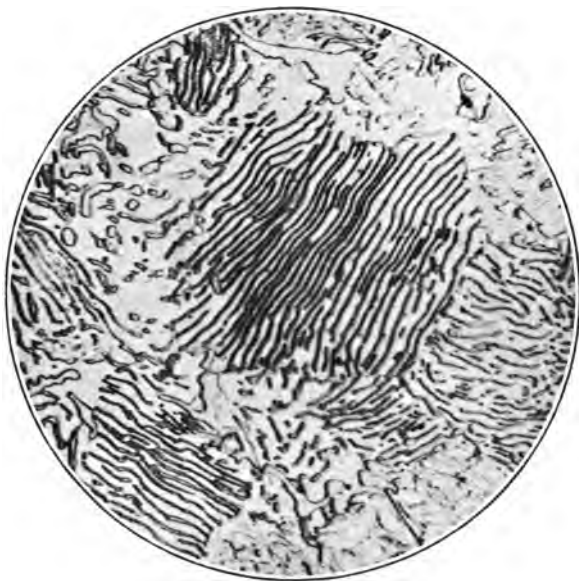
FIG. 25.—Pearlite. \times 1000 . [To face p. 164.]
