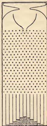
FIG. 72.—Galton's mechanical device for illustrating the law of the frequency of error, and the distribution of variates in the normal curve.
