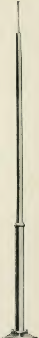
FIG. 112.—Iron pole with foot plate.
