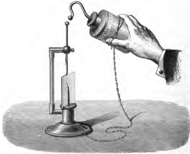
Fig. 399.—Puncture of Card.
