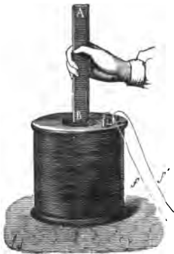
Fig. 544.—Current induced by Motion of Magnet.
