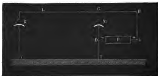
Fig. 530.—Principle of Caselli's Telegraph.
