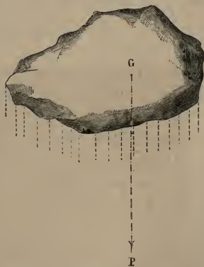
Fig. 18.—Parallelism of the Forces of Gravity on the different Points of a Body.
