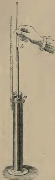
Fig. 126.—Proof of Boyle's Law for Expanding Air.
