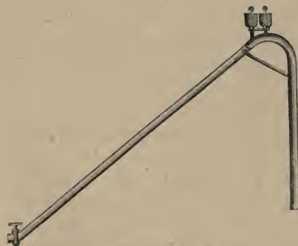
Fig. 178.—Siphon for Sulphuric Acid.
