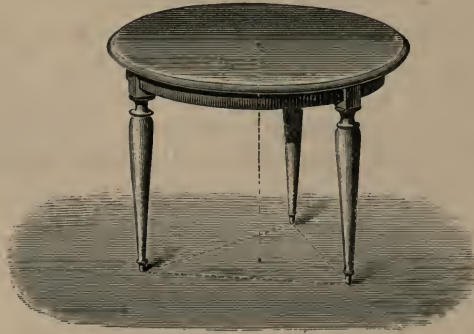
Fig. 25.—Equilibrium of a Body supported on a Horizontal Plane at three or more Points.
