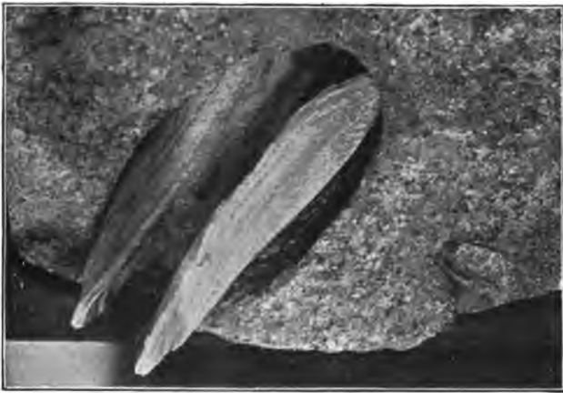
FIG. 105.— Dactylus sp., a mollusc, excavating granite. (Photograph by C. H. Snow; permission of Amer. Soc. Civil Engineers.)
