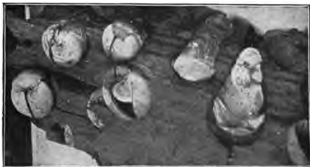
FIG. 107.— Martesia xylophaga , a Pholad, in Panama mahogany. (Photograph by C. H. Snow; permission of Amer. Soc. Civil Engineers.)
