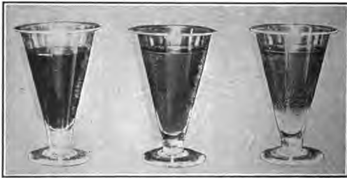
FIG. 50.—SEDIMENTATION GLASSES. A Clear. B, Slightly cloudy with beginning precipitation. C, Sedimentation complete.
