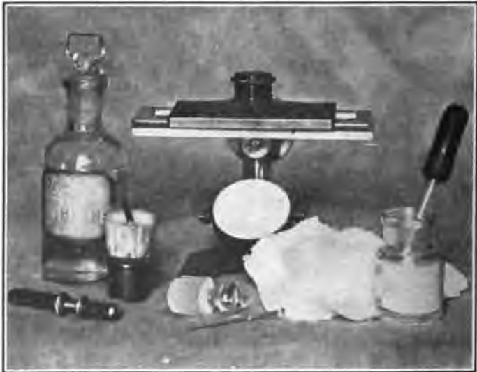
FIG. 9.—FLEISCHL HEMOGLOBINOMETER, SURROUNDED BY ACCESSORIES NECESSARY TO PERFORMANCE OF THE TEST, INCLUDING DALAND LANCET.
